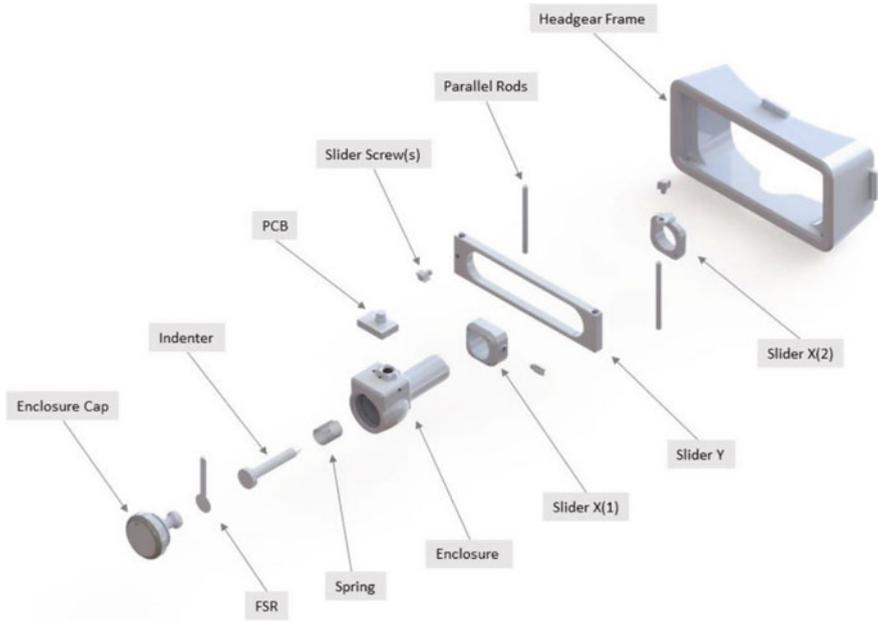
**Fig. 49.8** Exploded view of the device assembly
