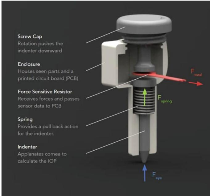
**Fig. 49.3** Placement of components inside the enclosure
