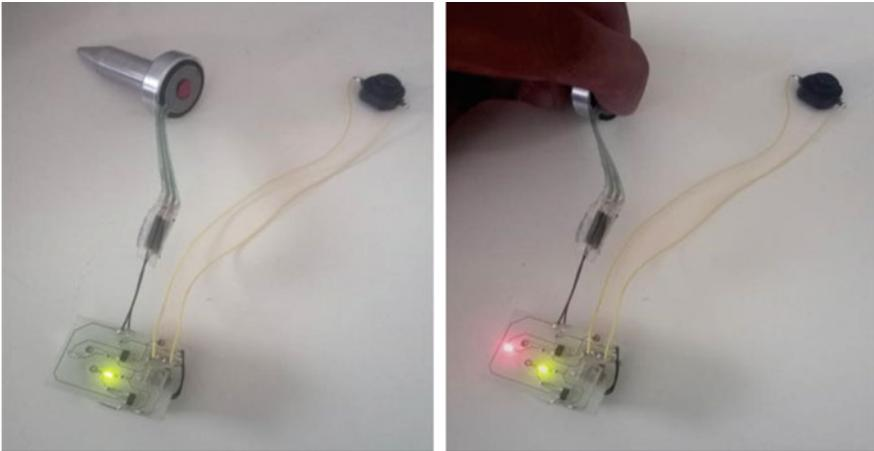
**Fig. 49.4** FSR without force (left), FSR with force (right)
