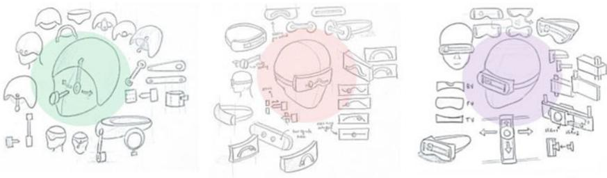
**Fig. 49.6** Ideation sketches of three concepts of the headgear: **a** Rotating (left), **b** fixed rail (middle), **c** linear (right)
