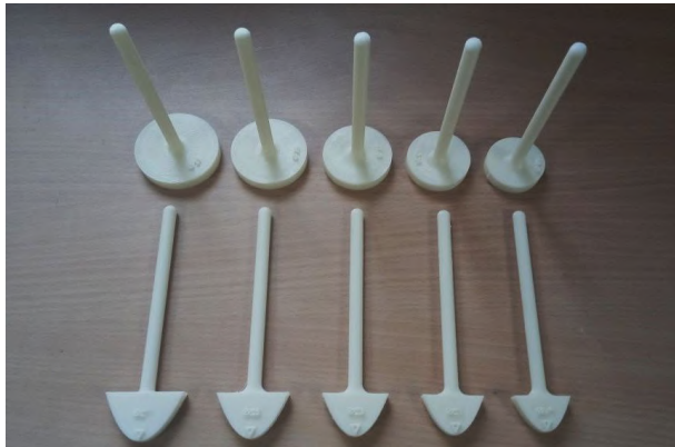
Initial prototypes made by 3D printing in biocompatible ABS-M30i
