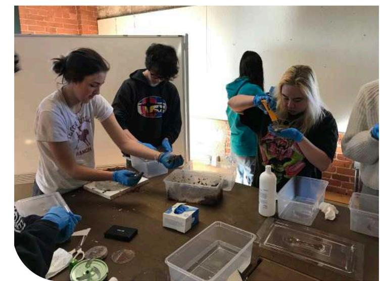
Participants packing molds with mycelium-waste mixture
