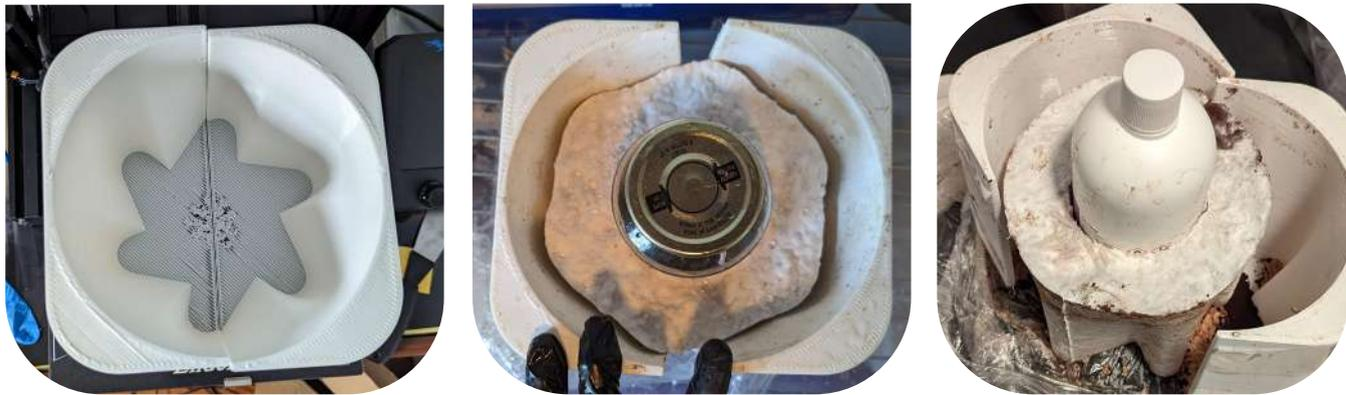
Used glass jars and old plastic bottles are used with two parts of the 3D printed mold to reduce the footprint of the process.
