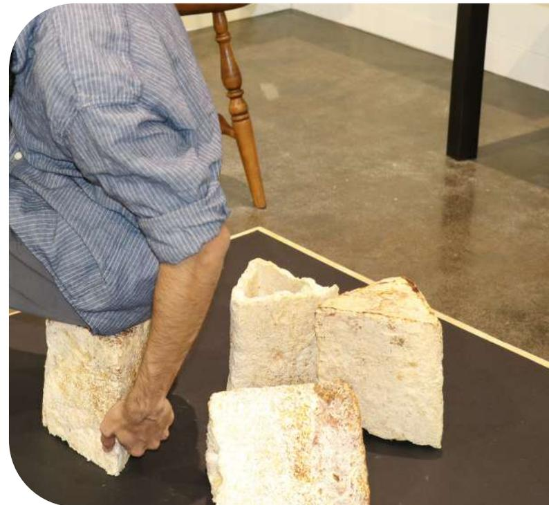
Three stages of mycelium module growth: cardboard and film, only film and open
