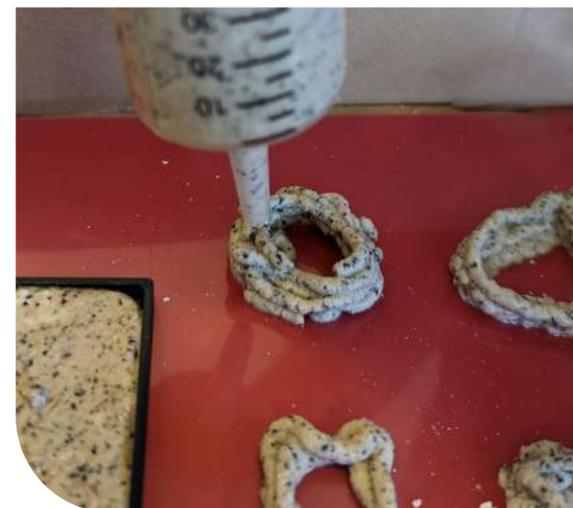
Manual extrusion experiments tested various compositions and paths for flow and adhesion of consecutive layers
