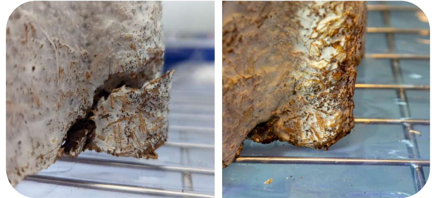
Mycelium has the ability to **self repair, heal and fix** disconnected areas and broken parts through its natural growth and binding process.
