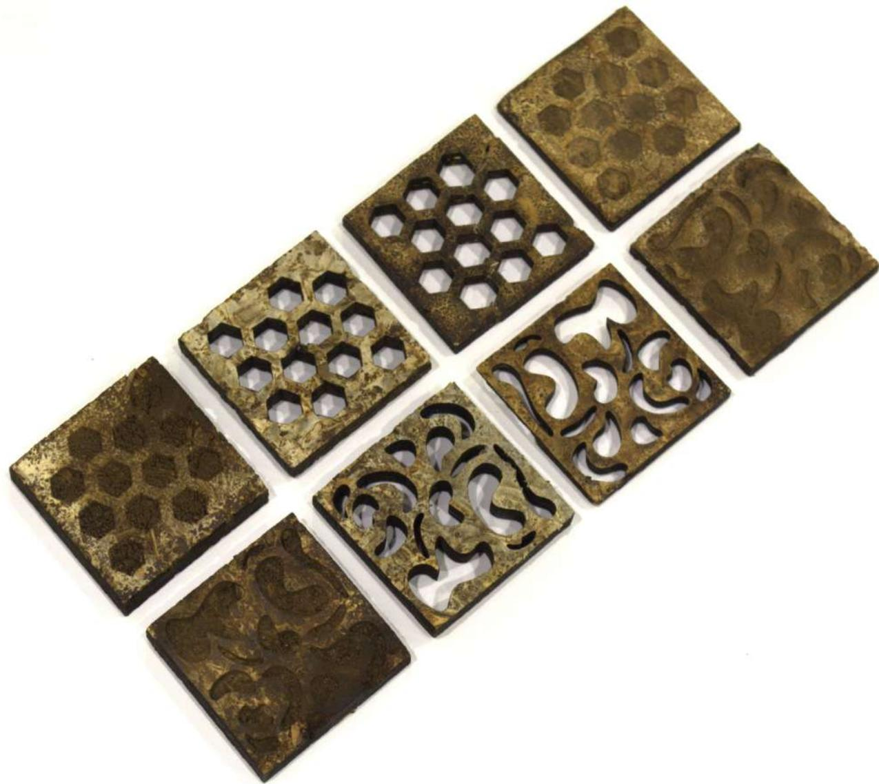
Laser cutting and raster engraving on myco-sheet samples at CoWorks Lab
