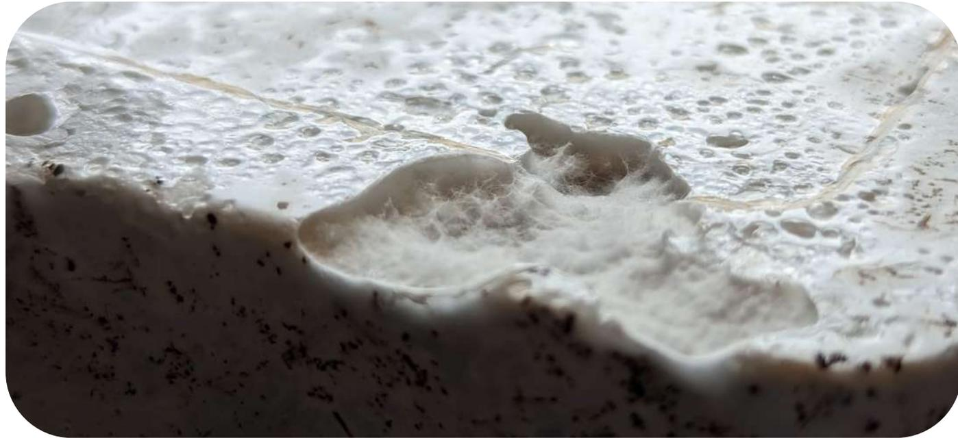
**Surface layers** of mycelium are maximized to 3 mm thick, improving structural integrity and surface texture
