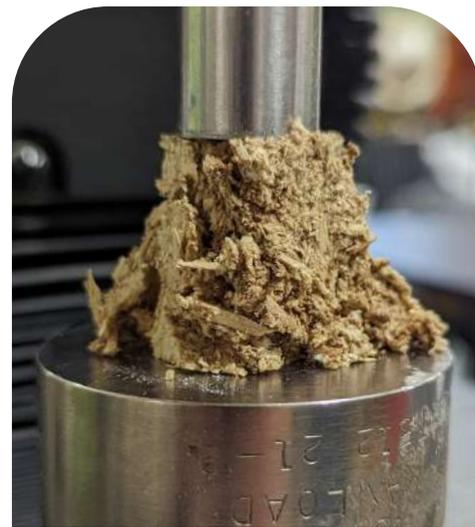
Myco-block sample compressed till failure in UTM at Brown Design Workshop.
